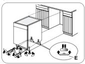
If necessary, pads (E) are supplied for the rear feet to make sliding the appliance in and out of the recess easier. To fit the pads, press them onto the rear feet.
